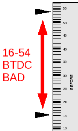
Timing marks on damper
