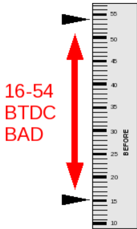
Timing marks on damper
