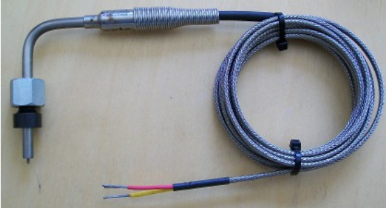
K-type thermocouple probe and bung.
