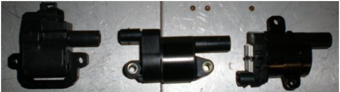
LS1 (left), LS2 (middle), Truck (right) coils
