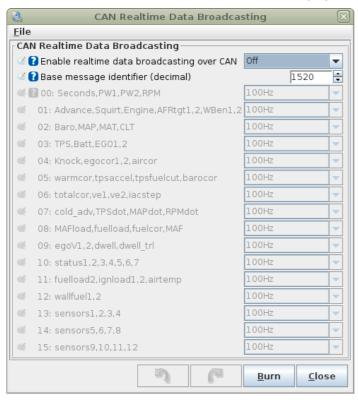
Once enabled, the user can select which data packets to broadcast and at what frequency. Be aware that the maximum capacity of CAN is around 4000 packets per second i.e. 40 channels at 100Hz. For reliable operation of other devices on the network it is suggested that a lower limit of 1-2000 be applied.
