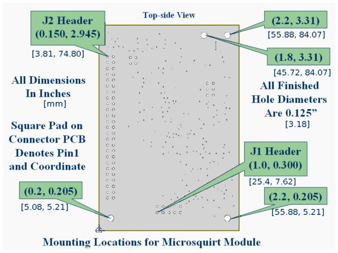
The two bolt holes on the top/right of the board are ideally used as additional heatsinking for the 5V voltage regulator.
